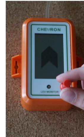
Hold a magnet to the right of the LED hole, approximately 10mm to the right of the LED, until the LED illuminates continuously. When this happens, move the magnet away from the Chevron and wait until the LED starts to flash. Once more, hold the magnet in the above position until the LED illuminates continuously. Now take the magnet away again. The website [www.monitair.co.uk](http://www.monitair.co.uk) has a useful video showing how this is done.
